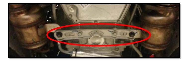
• Remove the secondary catalytic converter/factory X-pipe assembly
