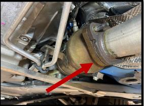
• Clean and deburr the cut edge on the remaining exhaust. This will ensure that the supplied barrel clamps seal correctly.
